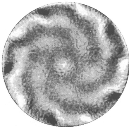
Fig. 4. - Shadowgraph image of the m = 5 state for \Omega = 2145 and \varepsilon = 2.6 . The entire pattern precesses in the rotating frame at constant velocity.
