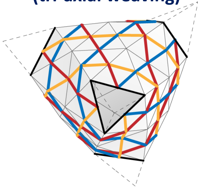
Kagome weaving (tri-axial weaving)
