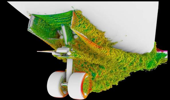
Flow field around the nose landing gear of a Boeing 777
